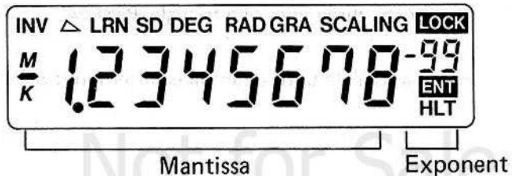
The Display shows input data, interim results and answers to calculations. The mantissa section displays up to 8 digits. The exponent section displays up to  $\pm 99$ .
